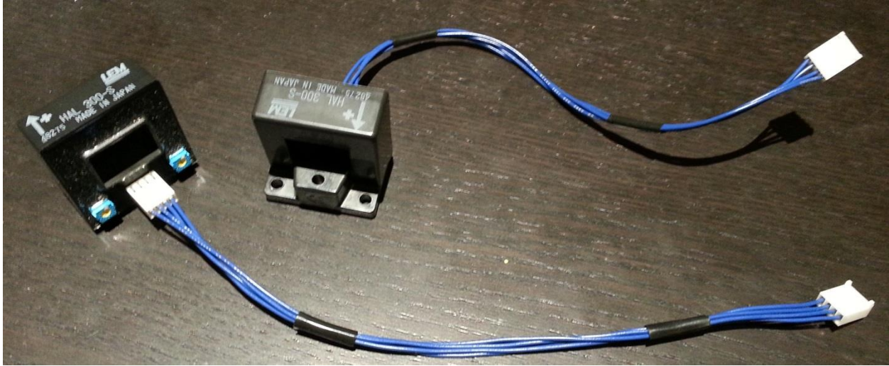
Figure 3: The HAL 300-S current sensors
